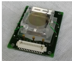
Figure 1: HinaLea Imaging's Solid-State Tunable Filter Production and the Model 4100H
